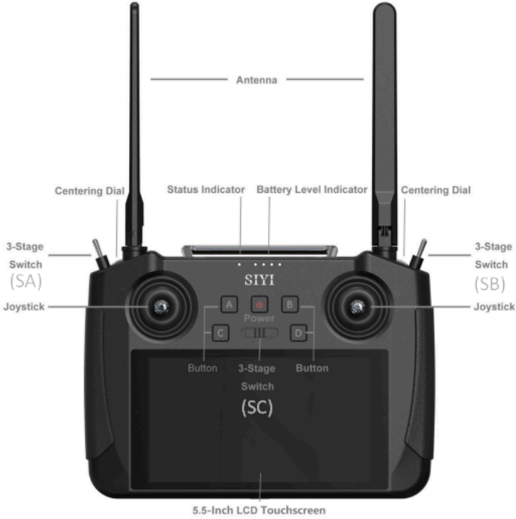
Figure 4.2.3: C2 Link Transmitter Nomenclature
