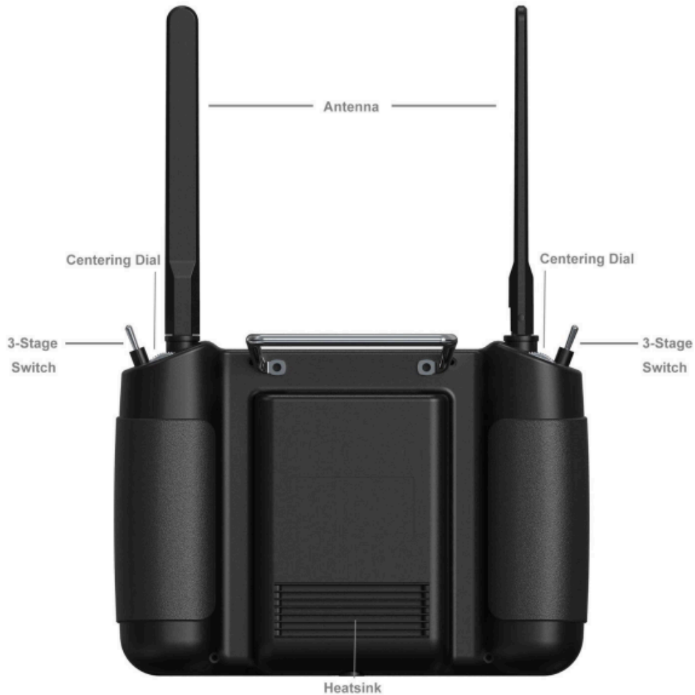
Figure 4.2.4: C2 Link Transmitter Nomenclature
