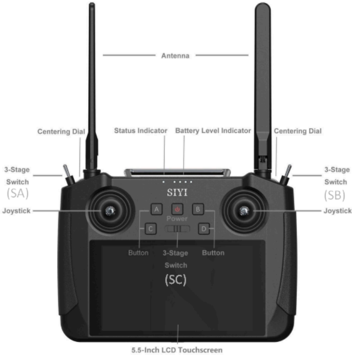
Figure 4.2.3: C2 Link Transmitter Nomenclature
