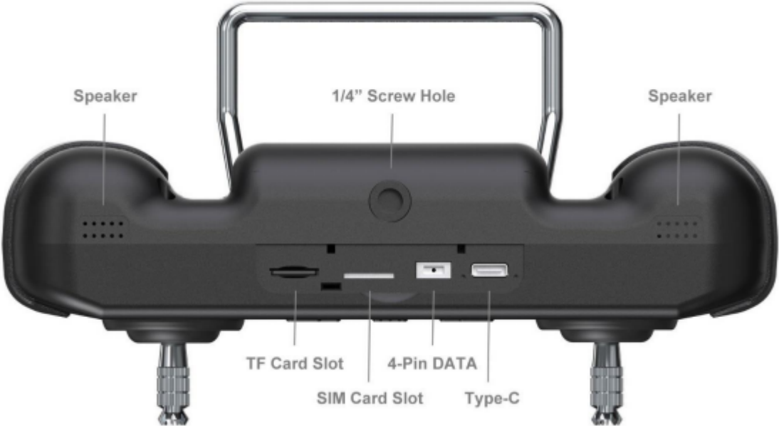
Figure 4.2.6: C2 Link Transmitter Nomenclature
