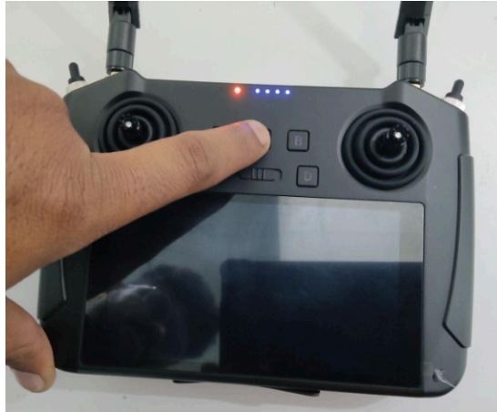
Figure 4.1.5: Turning Off the C2 link transmitter
