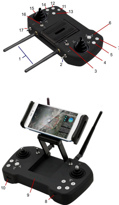
Fig 22: T12 Telemetry System
