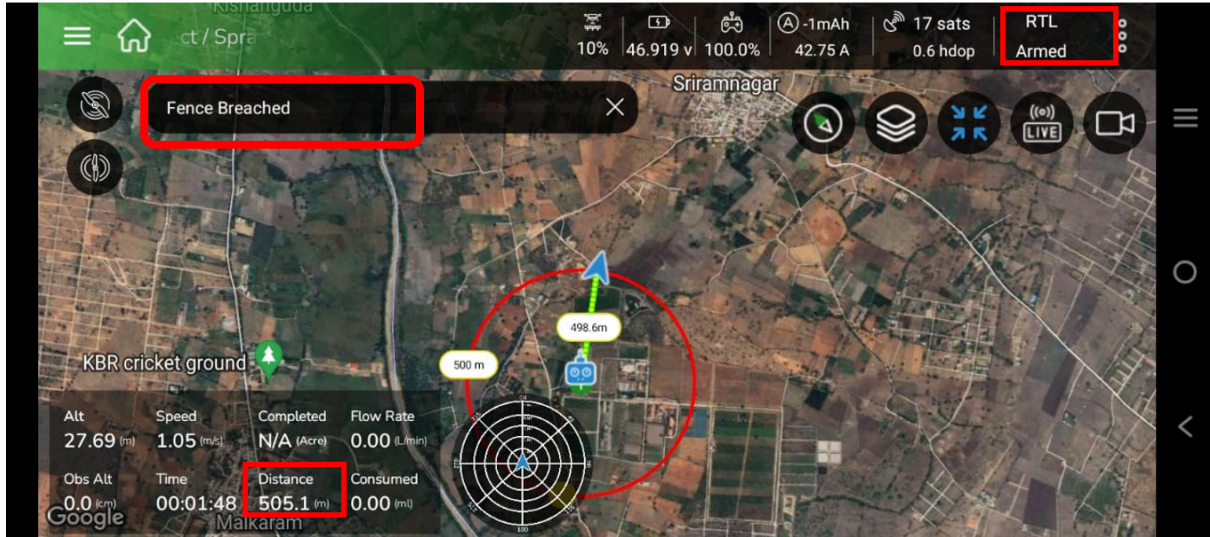
Figure : Shows the fence breach failsafe
